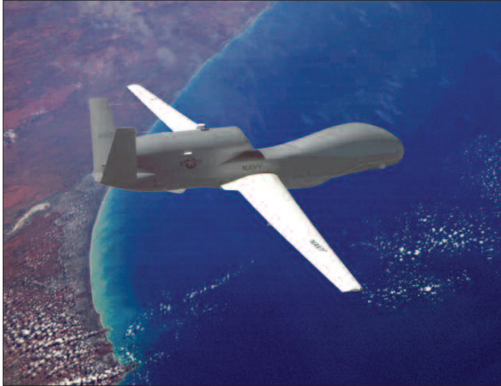
The high-altitude, long-endurance Global Hawk unmanned aircraft is well-suited to maritime surveillance missions.
