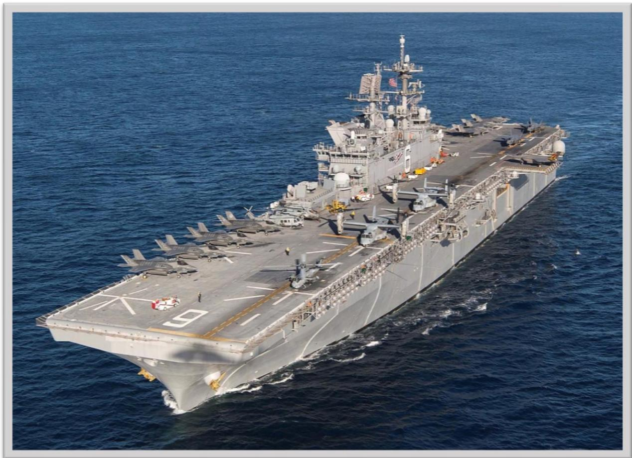
*USS America is lead ship in a new class of amphibious assault vessels that will serve as the centerpiece of future amphibious ready groups. Amphibious assault vessels are similar in size to the aircraft carriers of other nations, and are designed to host diverse combat aircraft, plus up to 1,687 Marines trained for amphibious operations.*
