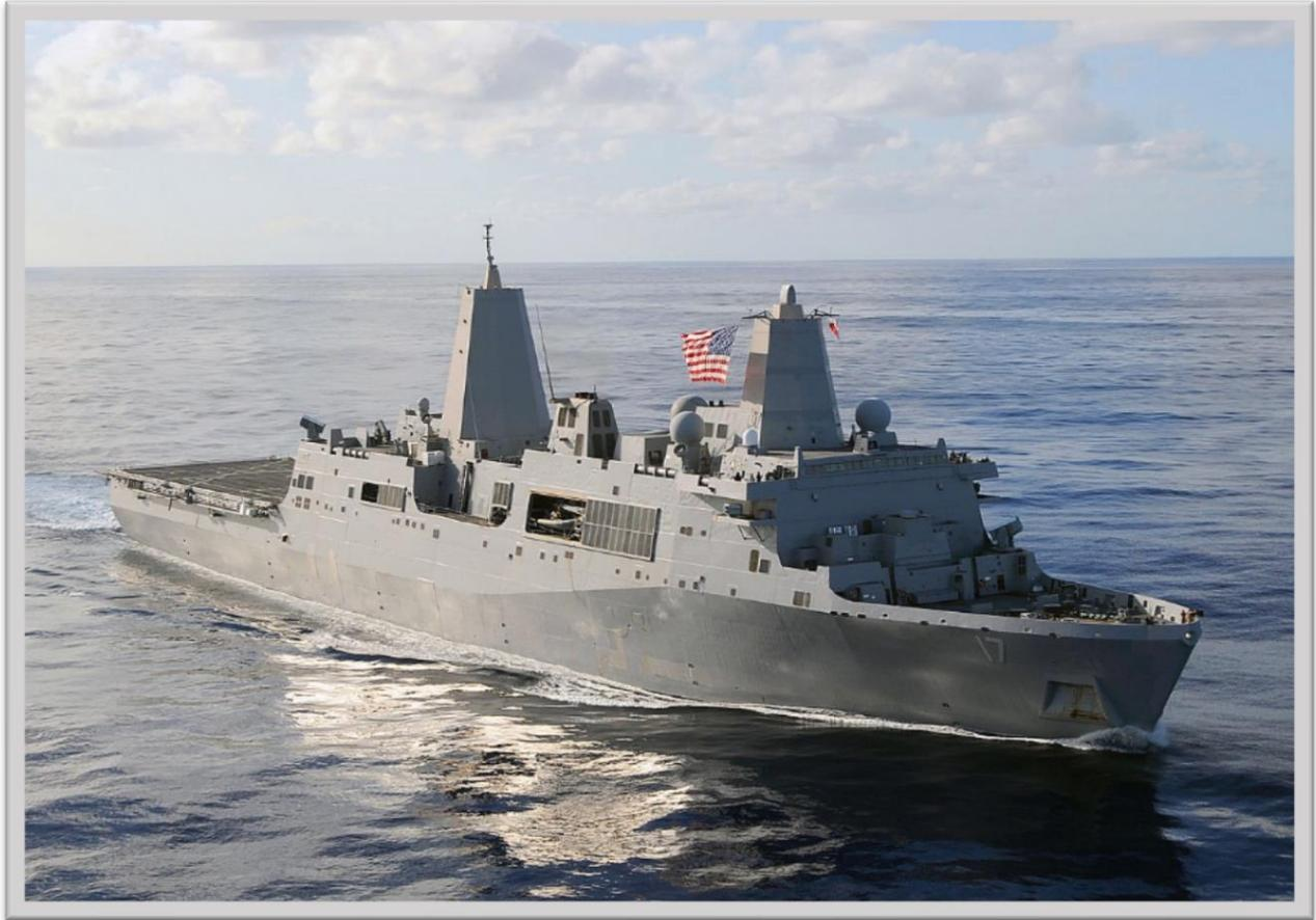
*USS San Antonio is lead ship in a class of amphibious transport dock vessels that each host 700 Marines and multiple rotorcraft. The unique configuration of the ship was designed to bolster survivability by deflecting hostile radar. A modified version of the same hull will be used to replace older dock ships, eventually comprising two-thirds of amphibious vessels in the U.S. fleet.*
