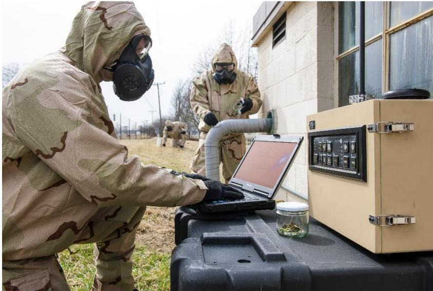
*A first responder uses the Resource Effective Bioidentification System (REBS) in a field exercise. Detecting and classifying dangerous pathogens or toxins is the vital first step in containing chem-bio threats. New technology such as REBS simplifies and accelerates that process so that countermeasures can be applied in a timely fashion.*
