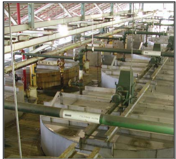
The Radford facility is unique in its ability to make nitrocellulose – an essential ingredient for propellants and explosives. There is no alternative domestic source for this material should an element of this process fail, such as the blenders pictured above.
