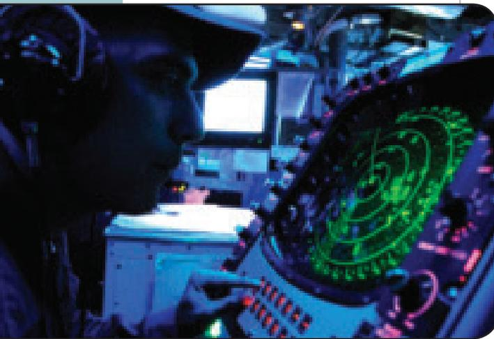
*Radar station in the command information center of the mine countermeasures ship USS Defender.*
