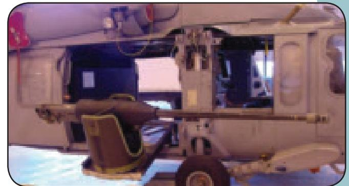
*The Rapid Airborne Mine Clearance System (RAMICS) will be included in LCS Mine Countermeasures Mission Package and deploy on the MH-60S helicopter.*
